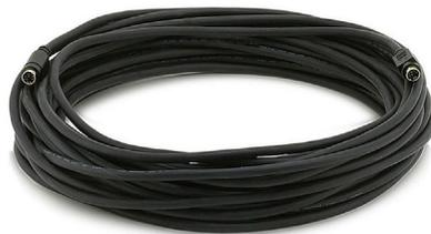
CASCADE cables are designed to daisy chain cameras to each other for the ability to control multiple cameras with a joystick or VISCA software. These male to male VISCA cascade cables include an 8-pin mini-din connector on each end. These cables are plenum rated. Available in black.
