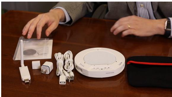
**Step 3:** Now it is time to charge your Wireless Speakerphone. A fully charged HuddlePod Air can operate for 7 hours of audio conferencing. Many times users will connect the included USB Charging Cable to a power source instead of relying on the battery power. When one end of the USB cable is inserted into the USB port on the device and the other end to the USB port on the computer or to a USB power supply, power
