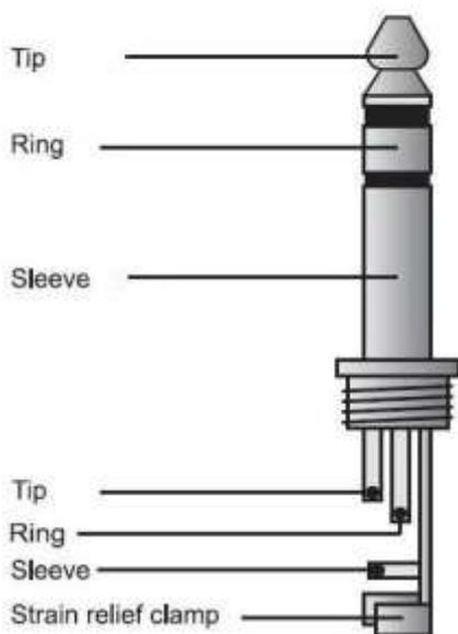
Connect the tip connector to the left (or mono) input of the amplification or recording device. Connect the ring connector to the right input of the amplification or recording device (or leave disconnected if input is mono). Connect the sleeve connector to the ground of one or both inputs of the amplifier or recorder.
