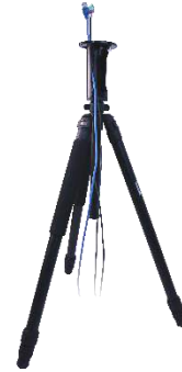
Route necessary cable through side opening in the column
