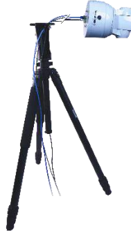
Connect all necessary cabling to the appropriate connectors on the base of the camera.
